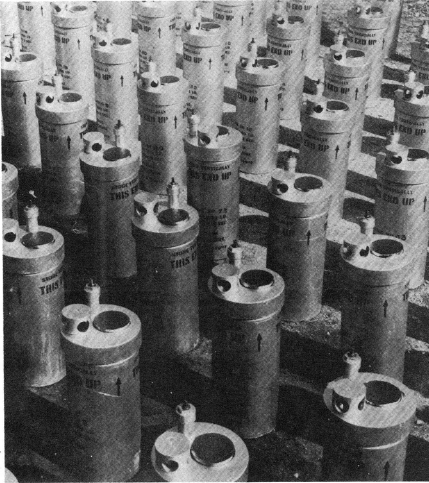
Figure 3 Typical Aerojet JATO units end-burning rockets using asphalt-based propellant.
